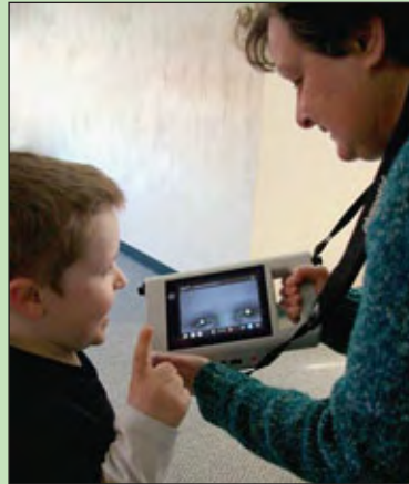
Blind & Vision Rehabilitation Services' vision screening technicians use a screening device that screens both of a child's eyes simultaneously in less than a second. The device provides immediate pass/fail results for a number of vision deficiencies.
